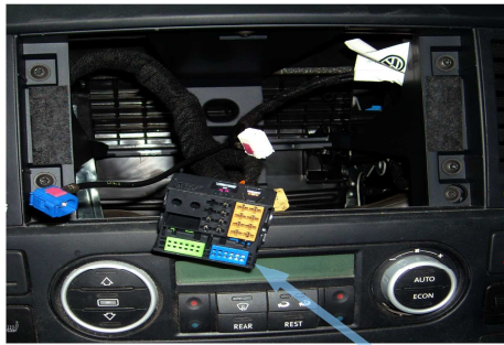
CAN-Abgriff am orig. Radiostecker Tap CAN on the orig. headunit connector
